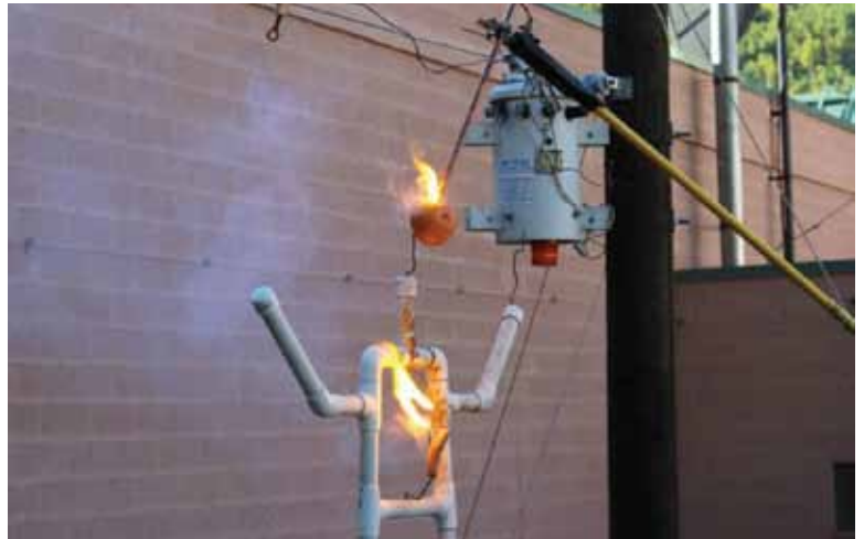
Above: Using a grapefruit to represent the head and a hot dog to represent the heart, SMPA's High Voltage Safety Demonstration simulates the effects on the human body when it comes in contact with a power line.
